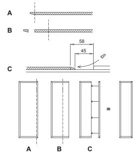
A. Cut off 13mm chamfer strip from behind and retain B. Reduce centre to its finished width less 13mm C. Attach reduced centre and chamfer strip to the trimmed wall panel to finish with a 45mm gap all round
